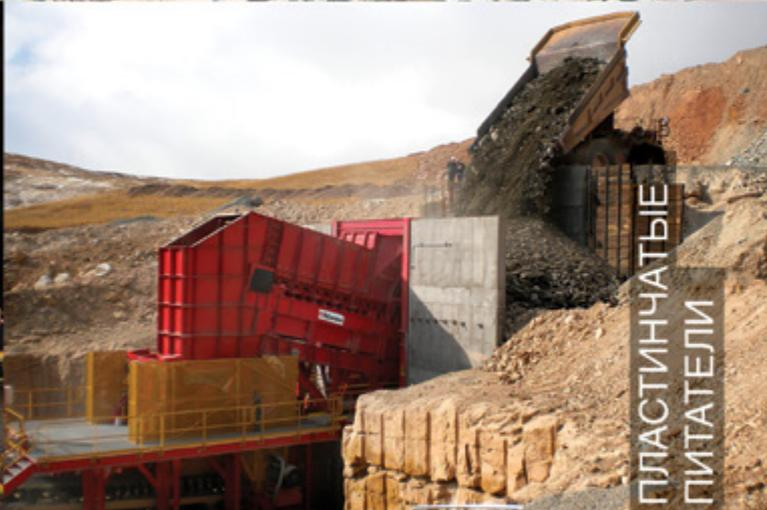
A red hopper-shaped feeder on a concrete base, with a conveyor belt leading to a large pile of material.
